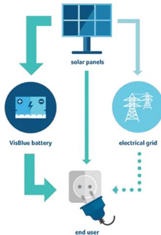
The VisBlue battery is an energy storage solution built around a unique Vanadium based Redox Flow battery. The VisBlue battery can store a day of solar energy, and power your home at night. With the Visblue battery the electrical power and storage capacity can be scaled independently. As the islands produce a growing amount of sustainable energy, storage on
